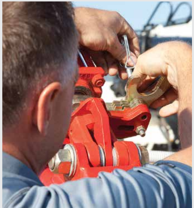
▲ shim pack design makes seed depth adjustment easy
